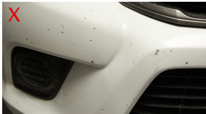
Excessive stone chipping
