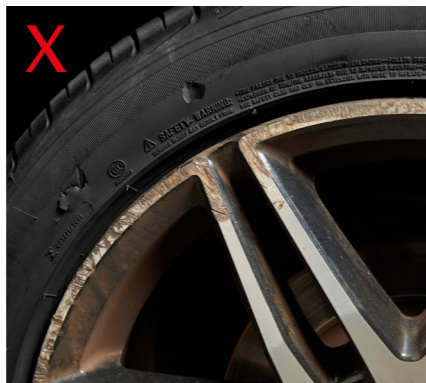
Excessive damage to wheels
