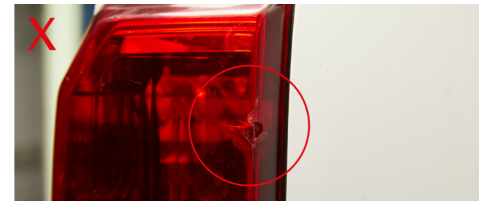
Cracked light cover
